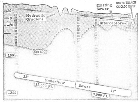
The new deep-tunnel sewer would be 12 feet in diameter on the west end and 17 feet on the east end. The present four-
