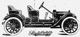
The Studebaker Flanders '29, with 100 inch wheel base, 4 cylinder, 20 horse power, 4 passenger car, complete with gas and oil lights, bonnet and magneto is the greatest car for the small price of
